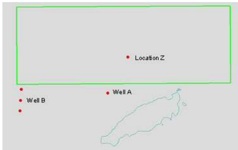
Fig 1. 3D survey area in green, nearest wells and possible drilling location red circles.
